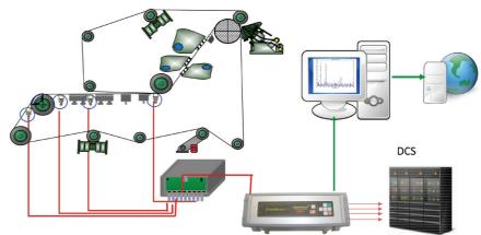
Figure 3. FiberScanFix system layout
