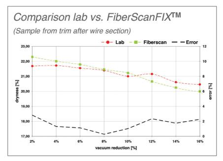
Figure 4. Laboratory vs measured comparison results
