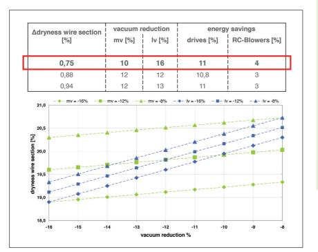
Figure 5. Vacuum reduction vs energy saving
