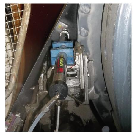
Figure 1. FiberScanFIX microwave sensor installation point in restricted areas
